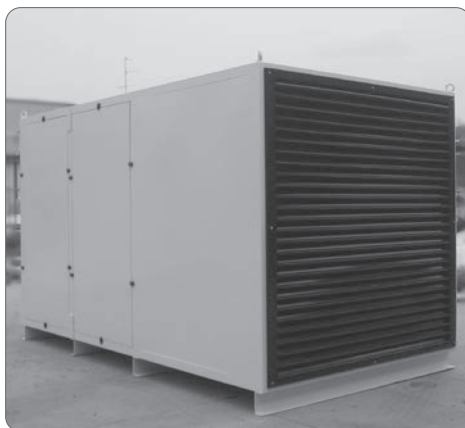
Centrifugal fan with afonic box, sound attenuator, inlet suction grilles with rainproof profile that can be opened for wall inspection G4 / G7 filter efficiency, multiple stages electric coil
